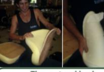
The seat and back components are stripped of foam and fabric. This process is facilitated by CGex technology, featuring a drawstring cut mechanism for easy release.
