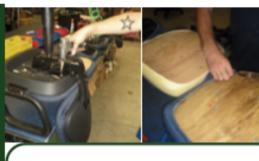
Each chair undergoes disassembly, separating it into its individual components including the base, gas spring, mechanism, seat, and back. STRIPPING PROCESS
