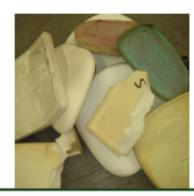
Foam waste is returned to Dunlop Foams which are then crumbed and used in high density carpet underlay and also as crumbed foam.
